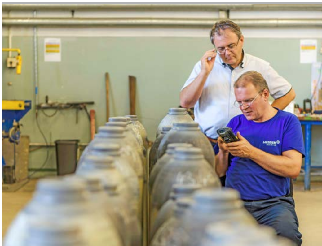
Up to 100,000 cylinders are tested at the modernised testing facility in Šal'a. Fótyi Dezider and Frantisek Tóth of Messer review the data with the aid of the BABEL system for cylinder tracking.
