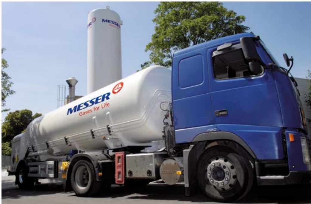
For customers with a greater demand for gases, Messer installs stationary tanks that are supplied by means of tankers.
